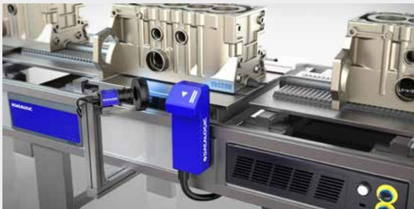
IMPACT Advanced OCR tool is able to effectively read serial numbers directly marked on automotive parts, even when surfaces are strongly reflective, rough and curved.
