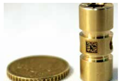
High contrast marking on highly reflective metal
