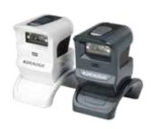
The Gryphon™ I GPS4400 is an on-counter, omnidirectional presentation scanner that offers hands-free scanning. It is the ideal size for space constrained environments and has an adjustable stand. It can also be used as a handheld reader for large or bulky items.
